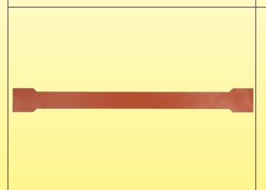
Type of sample tested (350 × 35mm)
