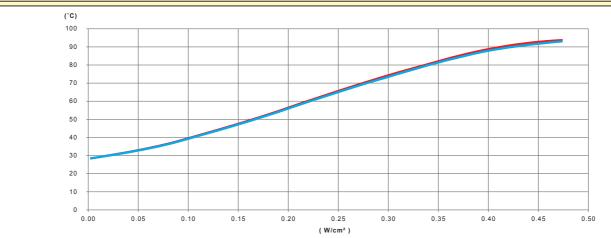
Variation, as a function of the power in W/cm² of the silicone heating ribbon, of the wall temperature of a galvanized steel tube filled with non-circulating water, thermally insulated by 20mm PVC-NBR foam
