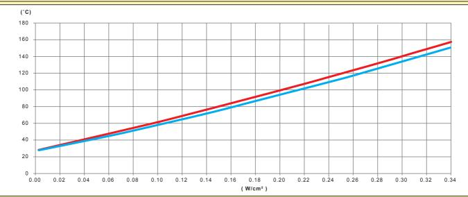
Variation, as a function of the power in W/cm<sup>2</sup> of the silicone heating ribbon, of the wall temperature of an empty stainless-steel tube, thermally insulated by 20mm of PVC-NBR foam
