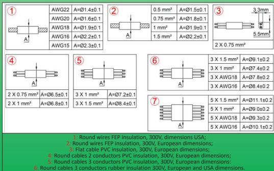
7: Round cables 5 conductors rubber insulation 300V, European and USA dimensions
