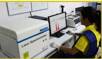
Spectrometric analysis in progress (Ultimheat Laboratory)
