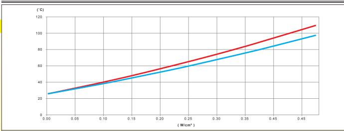
Variation, as a function of the power in W/cm² of the silicone heating ribbon, of the wall temperature of a stainless-steel tube, filled with non-circulated water, thermally insulated by 20mm of PVC-NBR foam
