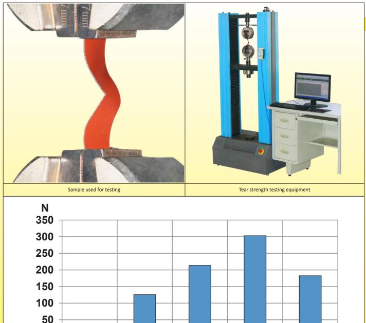
Comparative tear strength of the different thicknesses models 1: 0.8mm; 2: 1.6mm; 3: 2.3mm; 4: 3.2mm; 5: 2.3mm with stainless steel mesh reinforcement
