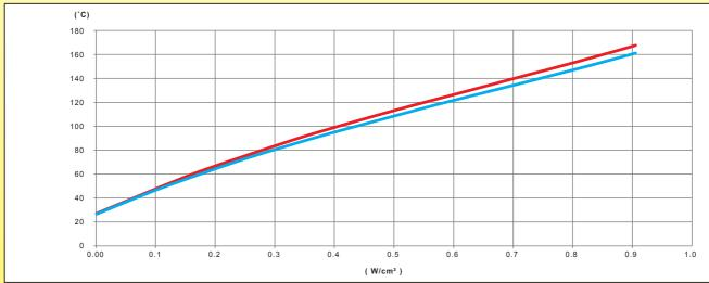
Variation, as a function of the power in W/cm<sup>2</sup> of the silicone heating ribbon, of the wall temperature of an empty, non-thermally insulated galvanized steel
