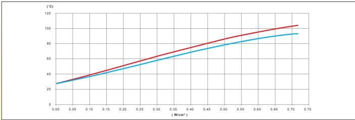
Variation, as a function of the power in W/cm<sup>2</sup> of the silicone heating ribbon, of the wall temperature of a galvanized steel tube filled with non-circulating water, non-thermally insulated
