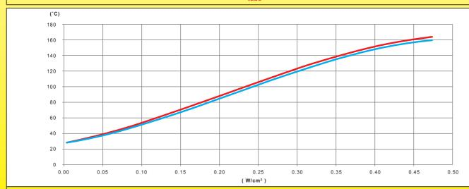
Variation, as a function of the power in W/cm<sup>2</sup> of the silicone heating ribbon, of the wall temperature of an empty, galvanized steel tube, thermally insulated by 20mm PVC-NBR foam
